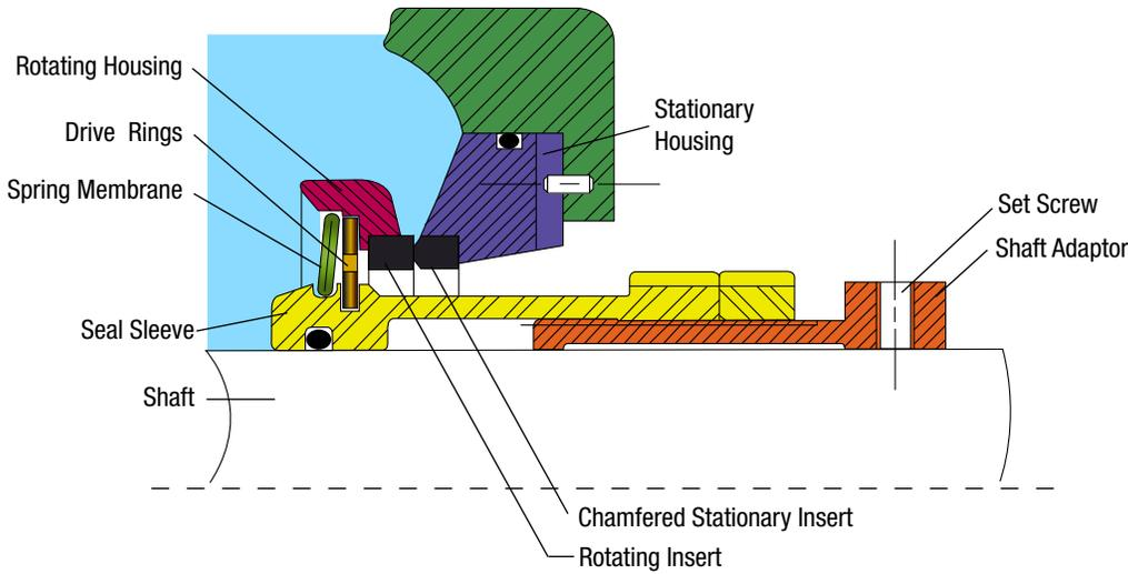
Chamfered face GPA® seal. This specific design has reduced seal face contact area resulting in lower breakout torque. Popular in latex paint manufacturing. Operating conditions are 100°F / 40°C, up to a 1000 rpm, pressure 30psi / 2.5bar.
