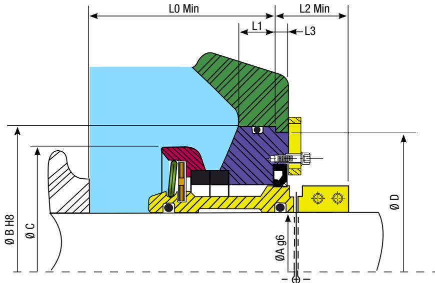
Style 43CP has a protected cartridge with the fixed ring on the impeller side. This design prevents dry friction and leakage of corrosive fluids. A lip seal is mounted in the fixed ring. Grease or flush water is used as barrier media.
