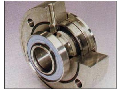
The GPEC is a cartridge type seal which has a built in ball bearing system. This provides excellent centering of the seal, since the bearing is very close to the friction surfaces.
