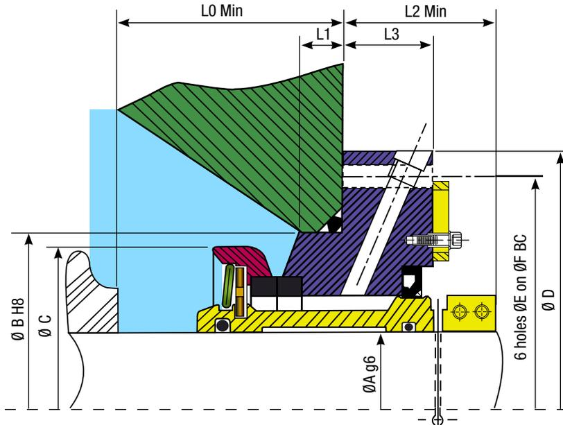
Style 03CP is a protected cartridge with the fixed ring installed on the drive side. This design is recommended for aggressive fluids; a lip seal is mounted in the fixed ring. Grease or flush water is used as barrier media.
