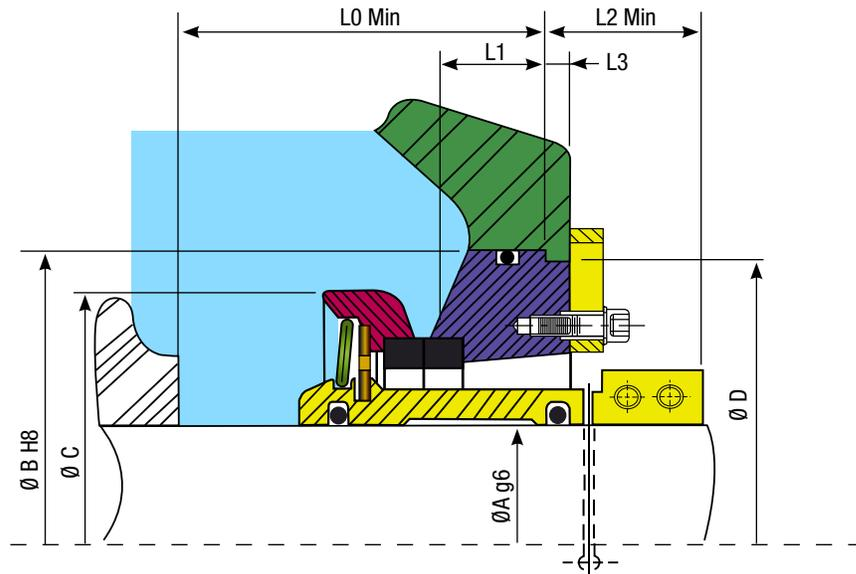
Style 43C is a cartridge seal with the fixed ring on the impeller side. These seals are preset at the factory. The characteristic table below lists standard sizes. Specific sizes are available upon request.
