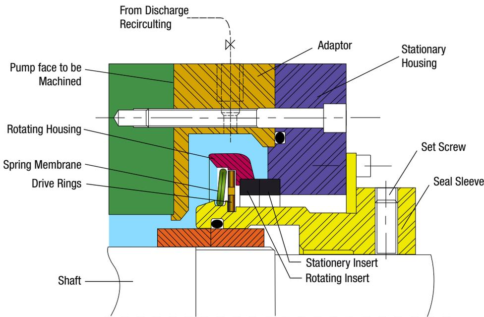
GPA® cartridge type, this specific design can be mounted outside of the pump body, in this particular case, operating at 200°F / 95°C, 1400 rpm, Suction pressure 25 PSI / 1.8 bar, discharge pressure 90 PSI / 6 bar. The seals replace the packing rings without modifications to the pump.
