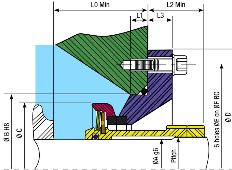
Style 03 is one of the most popular designs on the market. The fixed ring is installed on the drive side. The characteristic table below lists standard sizes. Special sizes are available upon request.
