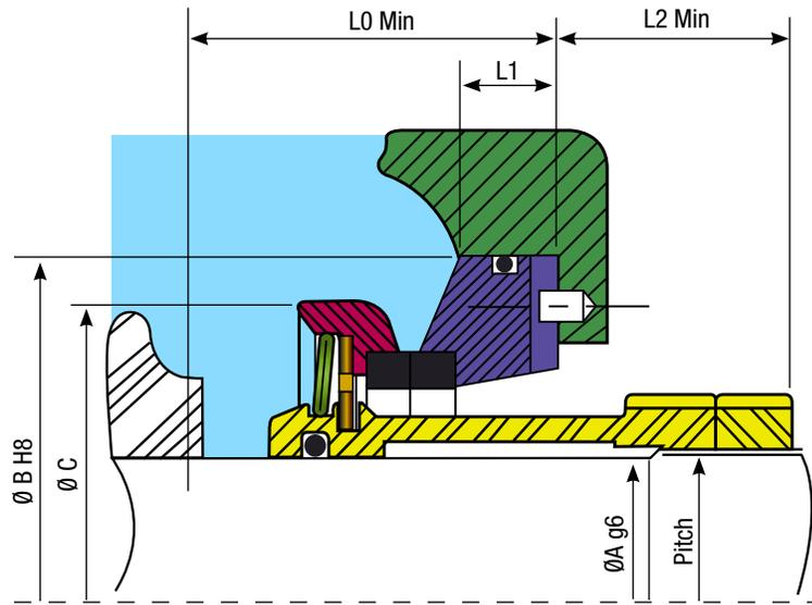
Style 13 available only in the threaded version is very easy to install. The fixed ring is mounted on the impeller side. The characteristic table below lists standard sizes. Special sizes are available upon request.
