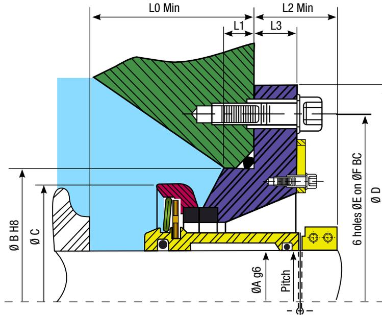
Style 03C is a cartridge seal with the fixed ring installed on the drive side. These seals are preset at the factory. The characteristic table below lists standard sizes. Specific sizes are available upon request.
