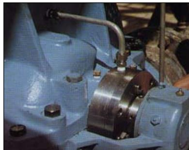
Double bearing external set up on 10LR pumps, Alumina processing, green liquor, Australia.
